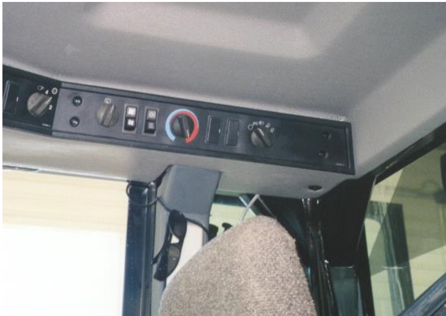
Switch panel and environmental controls on cab.
