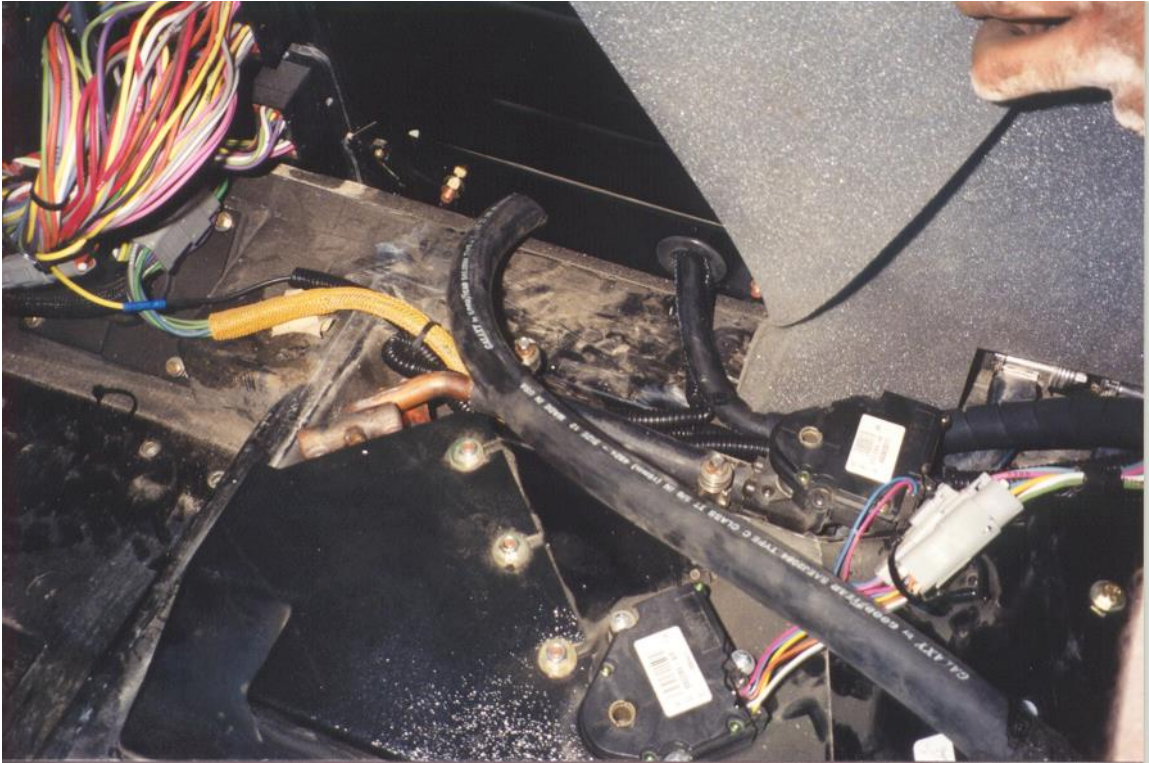
Hoses passing through hose plate (supplied) at rear inside of cab.
