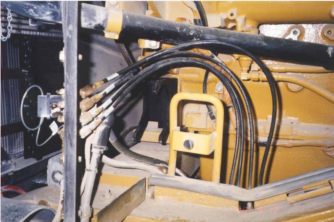
Compressor mount in place.
